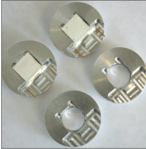
Fig. 6. Prototypes of p -terphenyl scintillation detectors for the MiRA_ep instrument
