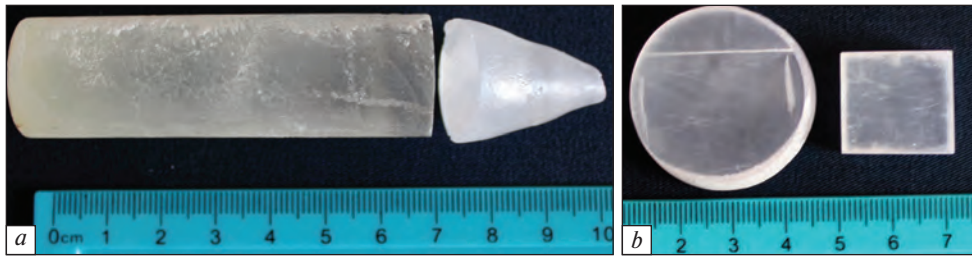
Fig. 5. An ingot of the p -terphenyl single crystal grown by the Bridgman method (a); a cylindrical workpiece of the p -terphenyl with the crystallographic axes' direction marking, and the p -terphenyl single crystal in a parallelogram form after mechanical treatment
